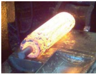
FORGING –Provides the BEST combination of mechanical properties
